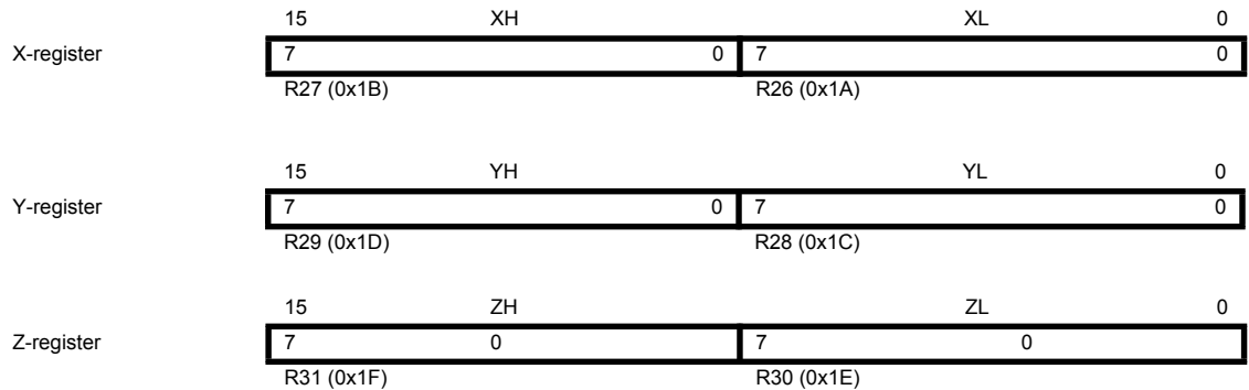
Figure 6-3. The X-, Y-, and Z-registers
